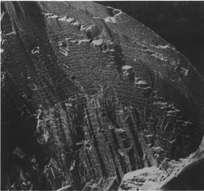
Figure 5 Fractured Supercooled Prill Showing Very Clearly the Dendritic Quasi Single Crystal Structure (S 6146)
