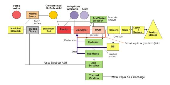
The critical chemical reactions in creating the Unity product take place in the Pipe-cross reactor. Only after the reaction melt exits the Reactor does the Unity process dry the material by relying on a combination of chemical thermal energy and combustion energy to remove water from the biosolids. This process results in a hard fertilizer granule that contains less than 2% moisture.
